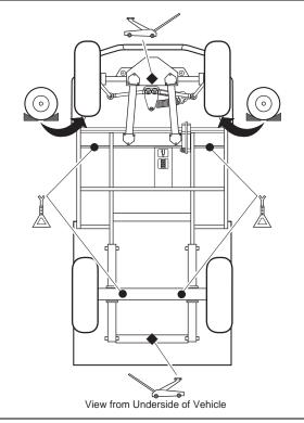
Fig. 16 Lifting the Vehicle
